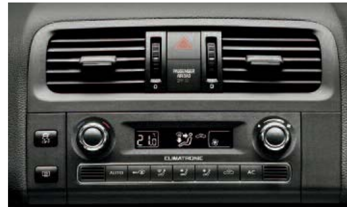
Climate Control Air-Conditioning
